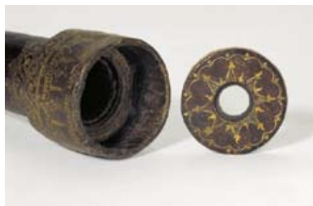
Detail of Telescope and objective lens. Galileo Galilei, Telescope, Florence, c.1610 Glass, wood, leather. Istituto e Museo di Storia della Scienza, inv. 2428
