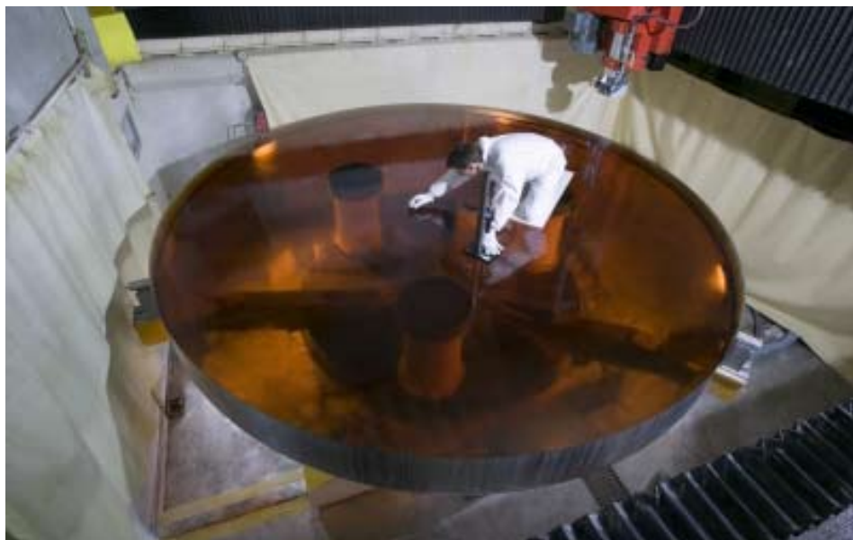
A technician inspects a 4-meter mirror substrate made of ZERODUR glass ceramic from SCHOTT AG in Mainz, Germany. The near zero-expansion material can be used in extreme operating temperatures without deviation in form, thus delivering crystal clear images for astronomical research. The material also demonstrates outstanding homogeneity, good chemical stability and can be precisely polished to meet the specifications for astronomical mirrors.
