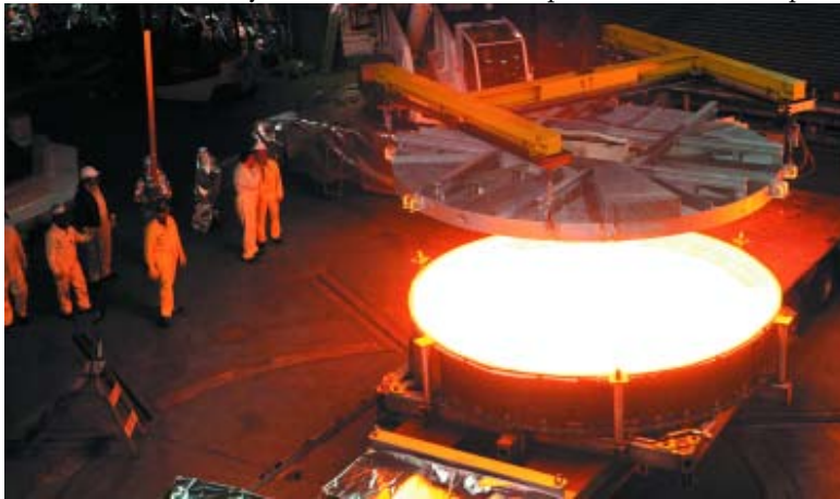
Casting of a 4 meter telescope mirror at SCHOTT made of ZERODUR glass ceramic at SCHOTT in Mainz. The casting has a temperature of over 1,000 degrees Celsius.
